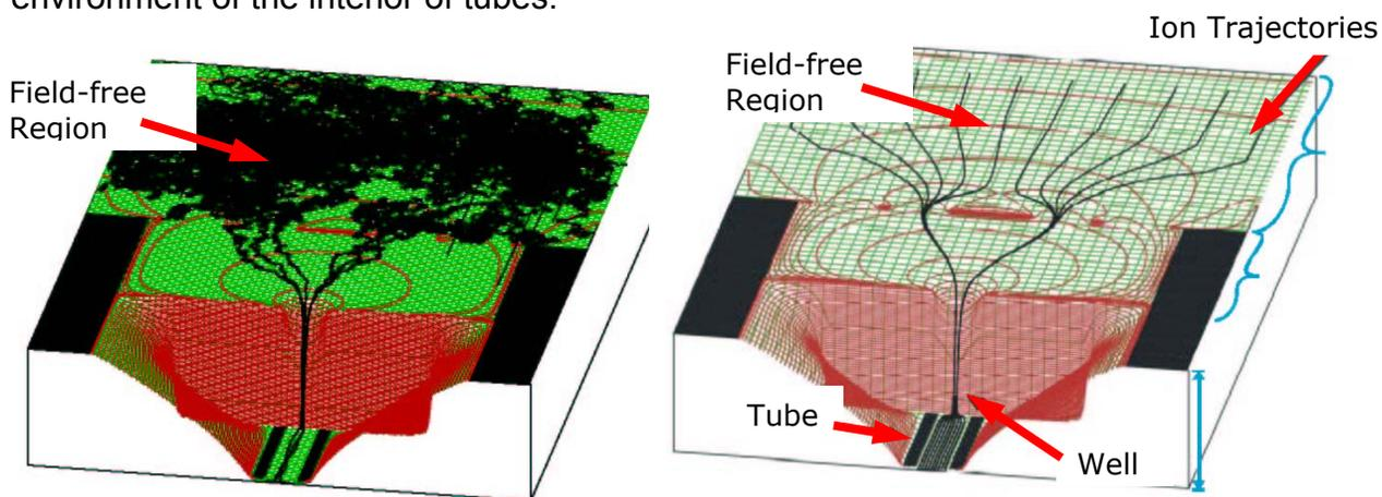
Figure 1 (left) The motion of ions in a field-free region is dominated by diffusion in the absence of electric fields or viscous flow of gases. (right) Simulation showing ion trajectories without considering diffusion.
